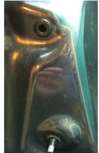
Now bumper is only held by clips. I found the best way to remove was to pull gently on the sides first to ease the top part free:
