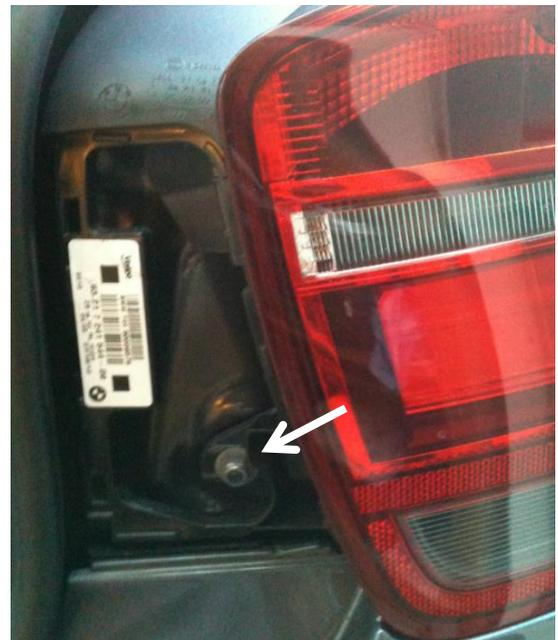
Light now pulls rearwards off 2 rubber fittings. This is tricky as you seem to need to pull quite hard. Try to ease it off the attachments carefully – it does come off, but be careful not to damage by pulling too hard on any one bit of plastic. Once off you reveal the fixings as shown. Disconnect cable and store light unit:
