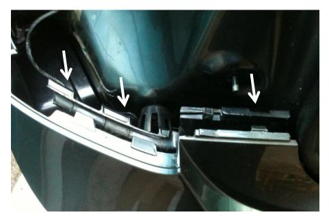
Once loosened, reach behind and detach parking sensor plugs and number plate light plugs. Put bumper aside.
