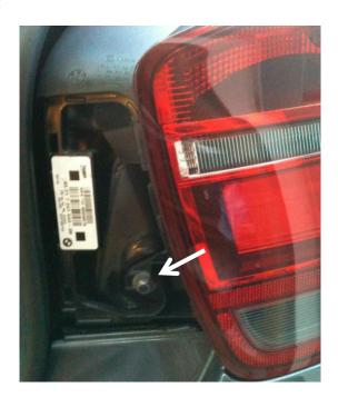
Light now pulls rearwards off 2 rubber fittings. This is tricky as you seem to need to pull quite hard. Try to ease it off the attachments carefully – it does come off, but be careful not to damage by pulling too hard on any one bit of plastic. Once off you reveal the fixings as shown. Disconnect cable and store light unit:
