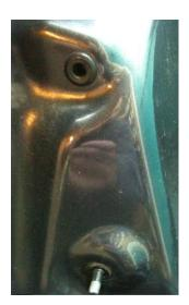
Now bumper is only held by clips. I found the best way to remove was to pull gently on the sides first to ease the top part free:
